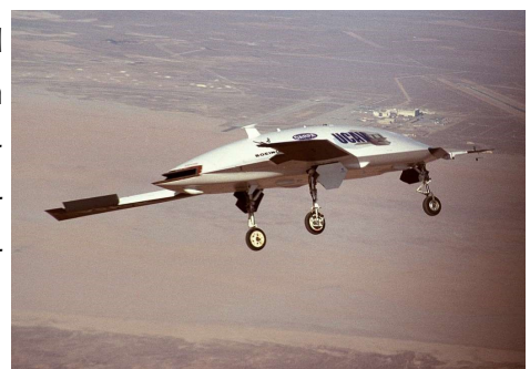
The X-45A, a stealthy, unmanned combat air vehicle that the Air Force hoped would play a role in the Vision Force.
